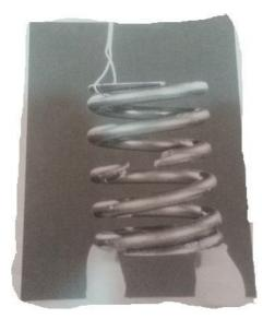
Figure 5.8: Broken Valve Springs
