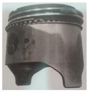
Figure 5.5a:Broken or worn piston rings
