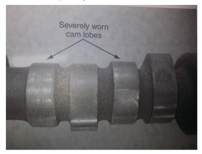
Figure 5.9: Worn Camshaft Lobes
