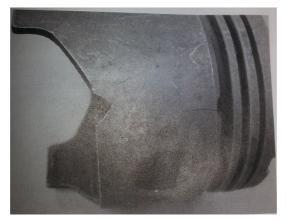
Figure 5.5b: Damaged piston
