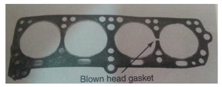
Figure 5.7: Blown Gasket
