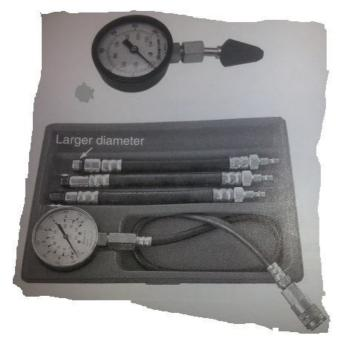
Figure 5.11a: Engine Compression Tester
