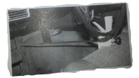
Figure 5.11b: A throttle depressor used to hold the throttle wide open during the compression test
