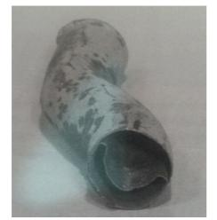
Figure 5.10: Collapsed exhaust pipe
